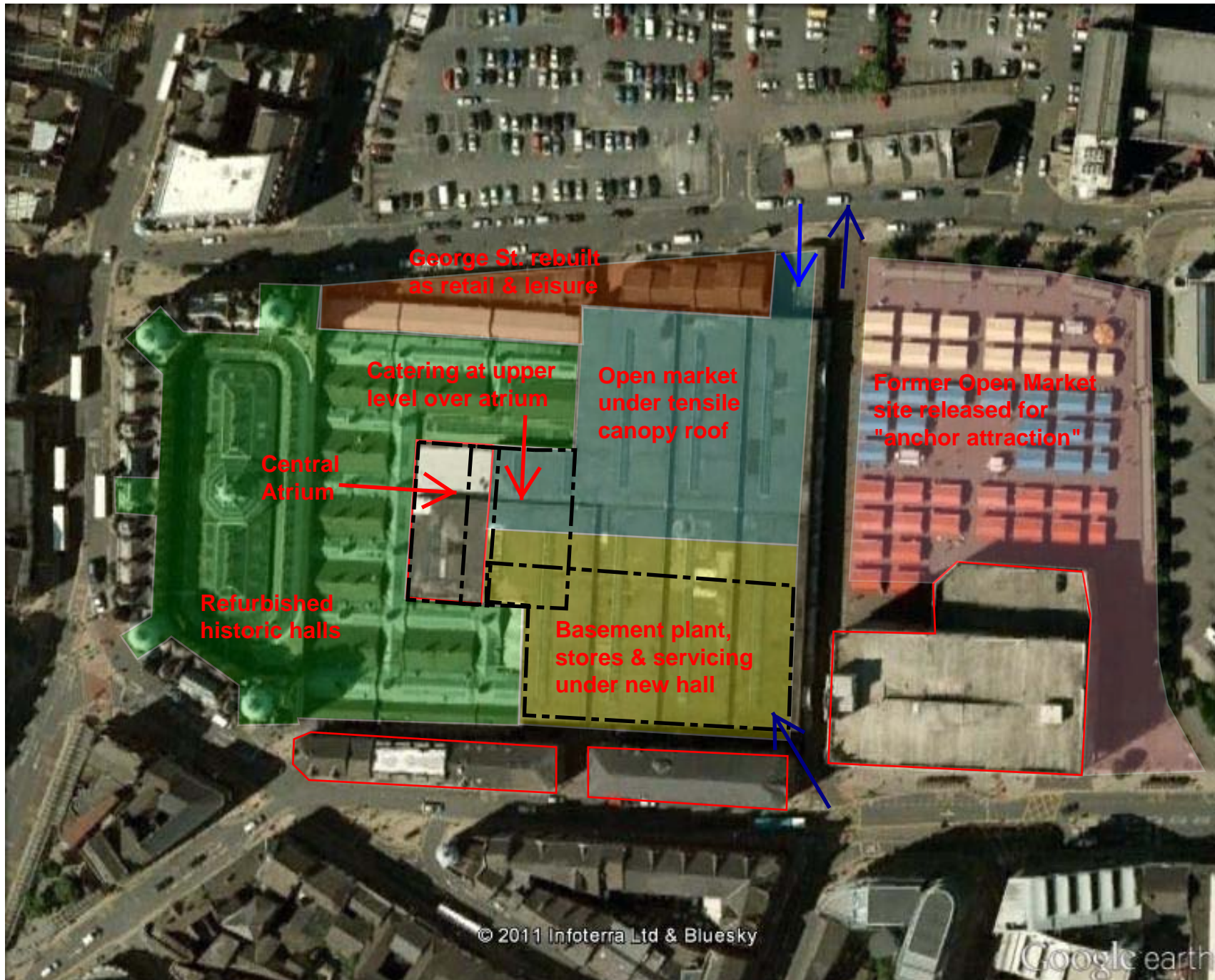
OPTION B: - NEW HALL + BASEMENT ON '76 SITE. DEMOLISH '81 HALL FOR NEW COVERED OPEN MARKET
